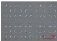
Raster printing results (Dot size : 5-7 \mu\text{m} )
